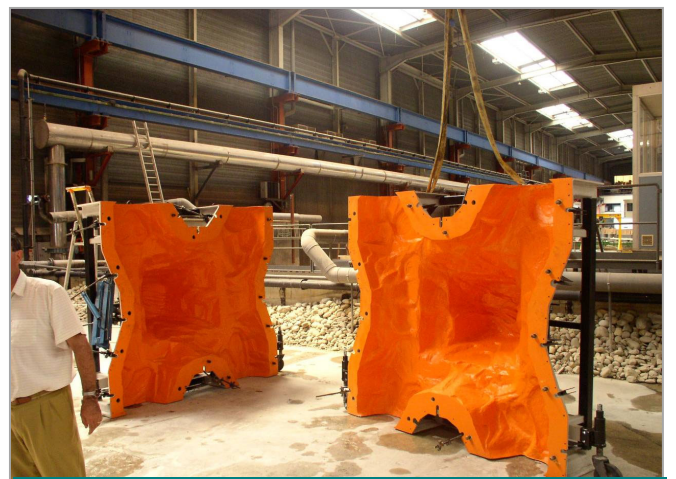
ECOPODE™ shells made of fibre glass
