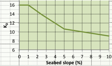
Graph 2: Relationship between the K_D stability coefficient and the seabed slope.
