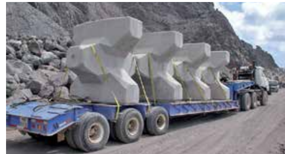
Hauling large units with a low trailer
