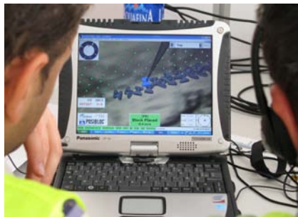
Figure 10. Underwater placement of first row of units
