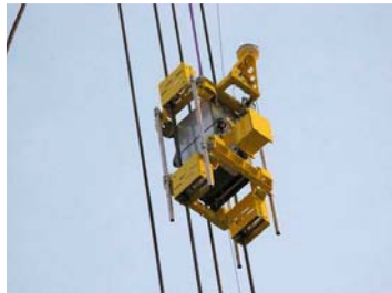
Figure 4. Cable drum measuring frame
